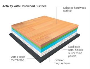
Harlequin Activity is a permanently installed sprung floor system, based on the well-established 'triple-sandwich' construction originated by Harlequin over 30 years ago. It's a fully floating system with no fixings to the sub-floor and can be laid on any reasonably smooth and flat surface without prior preparation.
