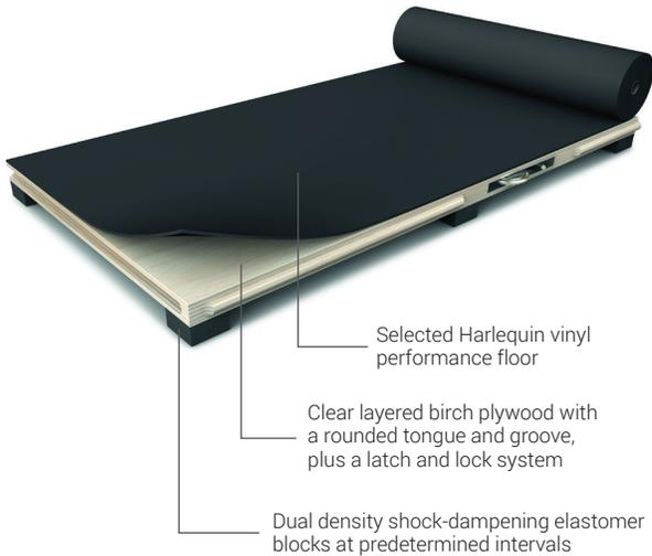
**Harlequin Liberty LatchLoc™** is a modular, sprung floor panel system manufactured from layered birch plywood featuring dual density elastomer blocks on the underside to give uniform and consistent shock damping. The panels are laid in a brickwork fashion onto the subfloor, so that cross-joins do not coincide. The panels join together by a rounded tongue and groove, which is secured in place using our 'one turn of the key' latch and lock mechanism.
